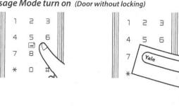
• Press PIN code or swipe KeyCard, then press "\*" within 8 seconds.
