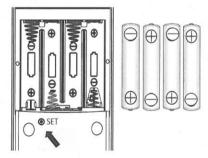
• Hold the "SET" button firstly and put batteries in until four "beeps" sound heard ( within 5 second ), then release the "SET" button.
