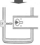
• Press end of the lever to open cover for unlock the door by key (even batteries run out).
